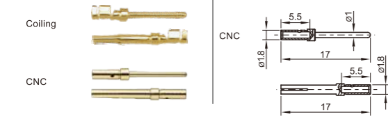
5A Female crimp contact For SF, SA, SP, SY, WP, WS/WF/WY16-28
